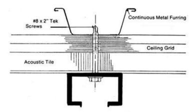
Method 2 - Attached to Wood wired or laid above the Acoustic Tile Grid
